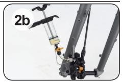
For bleed ports on the side, use the 90-degree syringe clip (F).
