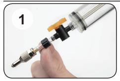
For brakes calipers that use a bleed nipple, begin by unscrewing the compression nut on one of the universal valves (B).
