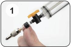
For brakes calipers that use a SRAM® Bleeding Edge™ fitting, begin by unscrewing the compression nut on one of the universal valves (B).
