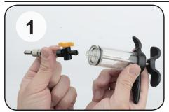
Assemble the syringe system by screwing the valve into the syringe. The valve comes pre-installed with a universal adapter that is compatible with many common hydraulic disc brake calipers and levers.
