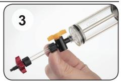
Install the adapter hose for Bleeding Edge  $^{\text{TM}}$  (I) onto the valve nipple and tighten the compression nut to secure it.
