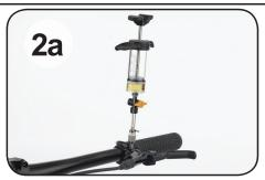
For levers and calipers with bleed ports on the top, use the upright syringe clip (E).
